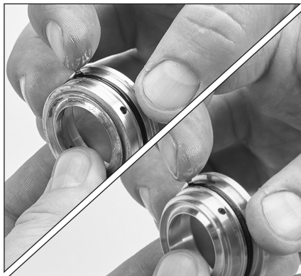
1.43 Replace seal case O-ring with new one from seal kit and apply a lubricant to outside surface.
