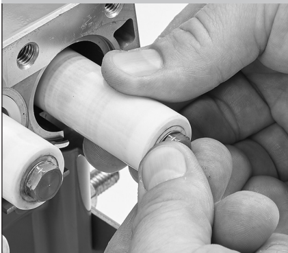
1.38 Thread plunger assembly into plunger rod by hand, and torque to 55 in-lbs, 4.6 ft-lbs or 6.2 Nm.
