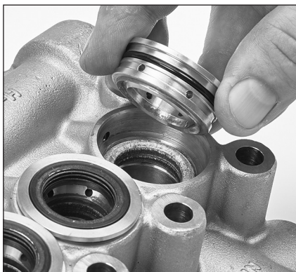
1.44 One side of the seal case has a groove. Install groove side facing down into the manifold and press into place.
