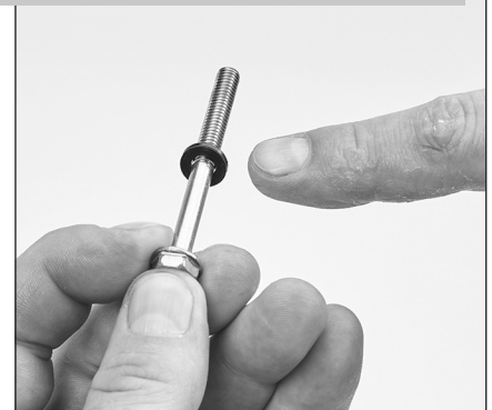
1.24 Remove and inspect seal washer.
