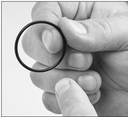
1.10 Inspect the seal case O-ring for cuts, nicks or damage.
