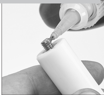
1.37 Place a drop of Loctite® 242® on the threaded end of the plunger rod.
