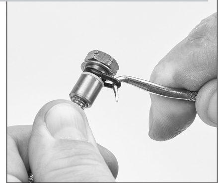
1.21 Using a pick, remove the plunger retainer O-ring from plunger retainer.
