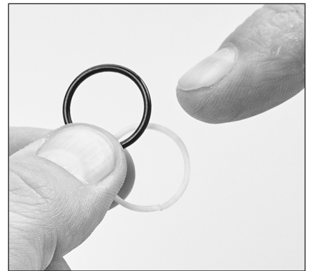
2.12 Inspect valve seat O-ring and backup ring for cuts, nicks, or damage.
