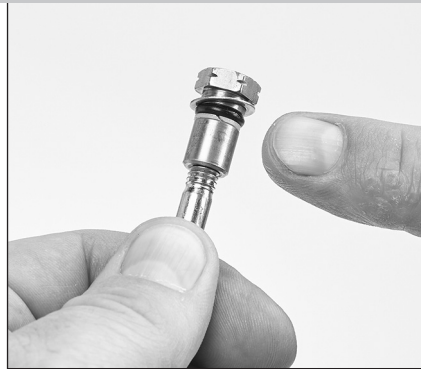
1.20 Remove the plunger retainer from the plunger and inspect the O-ring and backup ring for damage.
