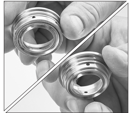
1.11 Inspect the grooved V-packing surface of the seal case for scoring or damage.
