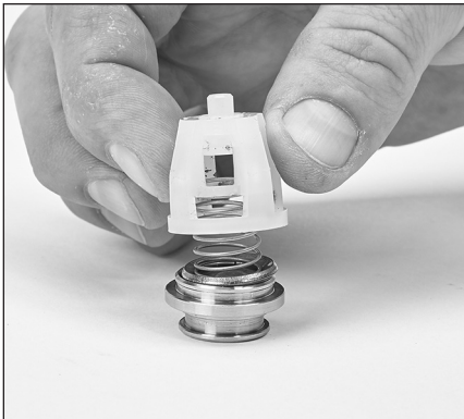
2.16 Place spring retainer onto valve seat.
