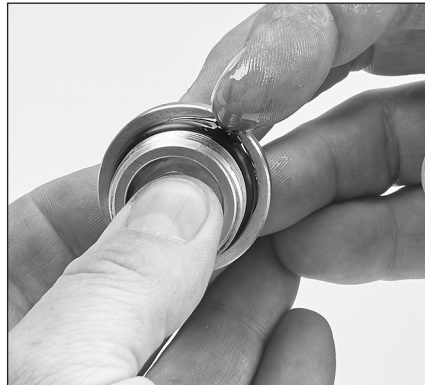
2.21 Replace valve plug O-ring with new one from valve kit and apply a lubricant to outside surface.
