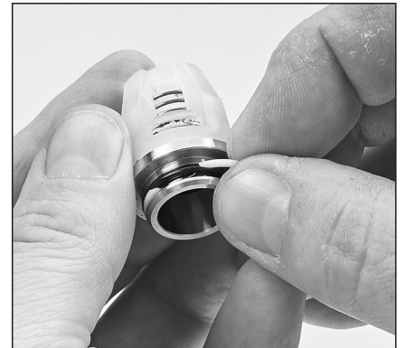
2.18 Replace valve seat O-ring into the top of the groove, then backup ring at the bottom.
