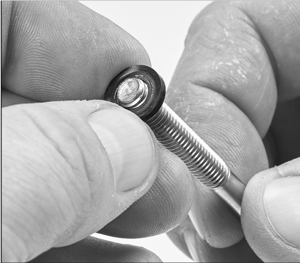
1.33 Replace seal washer with new one from seal kit.
