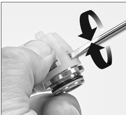
2.05 Insert flat tip screwdriver through spring retainer just above valve. Twist to create a small gap between valve retainer and valve seat.
