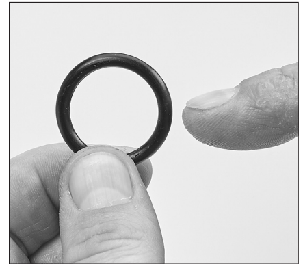
2.03 Inspect valve plug O-ring for cuts, nicks or damage.
